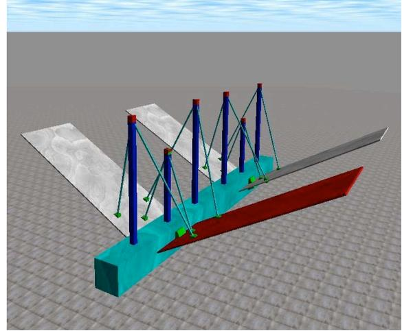
**Figure 0. Cable Actuated Model. In practice cables extend symmetrically below wing and close a loop.**
