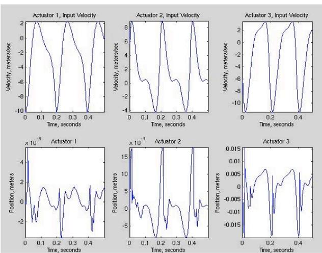
**Figure 4.** These graphs show the fully evolved pattern of input velocities and the resultant positions of the actuator joints over time.
