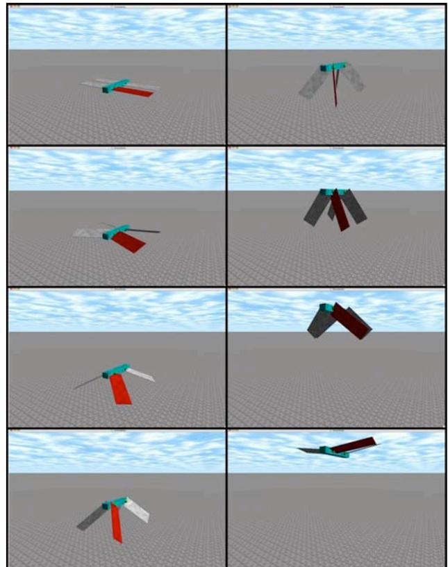
Figure 3. This image sequence shows one cycle of the evolved flapping pattern (top to down, left to right).
